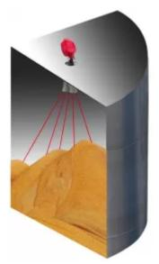
This illustration shows material piled unevenly in a silo segment and how the 3DLevelScanner measures mul- tiple distances across the material surface to account for irregularities when calculating volume.
