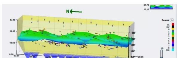
In this screen image, the topography of material is displayed and used to detect level per section.
