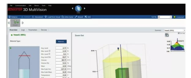
It is evident from the 3D graphic that material is disbursed evenly and the cone is up. The average, minimum, and maximum levels are displayed along with the volume and mass.
