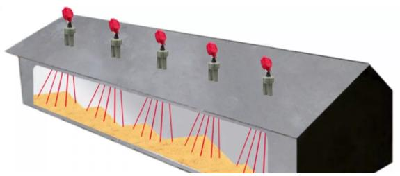
Several 3DLevelScanners are strategically mounted on the roof with each scanner measuring multiple points in a 70-degree beam angle.
