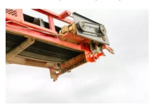
The Martin® SQC2S™ Secondary Cleaner removes dust and fines in scratches and divots not cleared by the primary cleaner.
