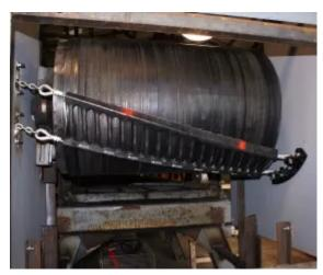
The CleanScrape® cleaner takes up minimal room and requires less maintenance than standard cleaners.
