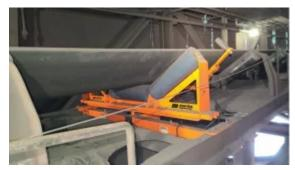
The torsion rollers ride smoothly on the belt edge, detecting slight variations in the belt path.
