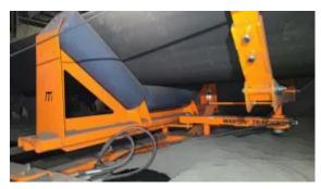
The pivoting idler assembly rotates in the opposite direction of the mistracking belt.
