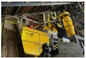
A STEINERT CHUTEC chute sorter uses X-ray fluorescence technology for sorting fine heavy metals with grain sizes down to 5mm. (Pictures: ©STEINERT GmbH)
