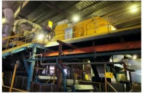
Several STEINERT KSS multi- sensor sorting systems with X-ray transmission technology generate high-purity aluminium products.
