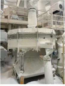
Before the switch to BFM® fitting, the customer experienced a lot of dust and material loss from their sifters. (Pictures: ©BFM® fitting)
