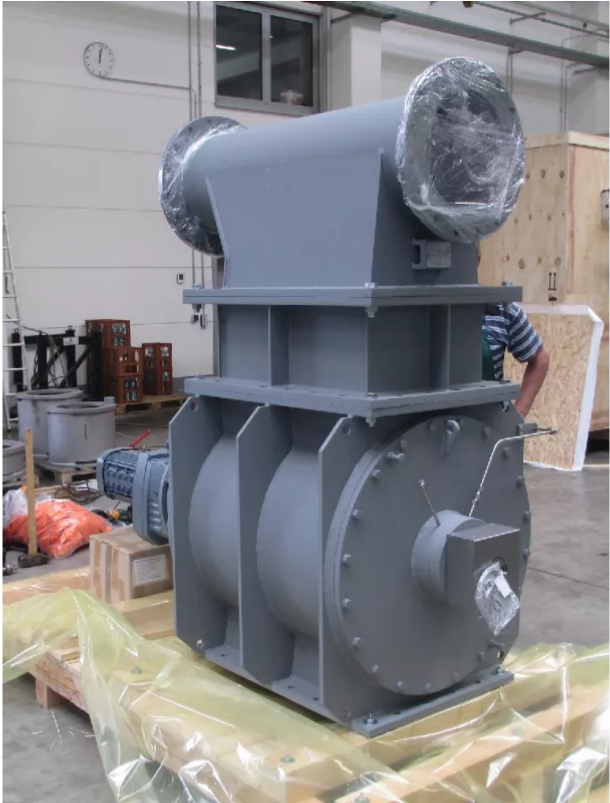
Fig. 3: KREISEL Ceramic rotary feeder Type 700x700-11 LU with mounted leakage air collector and with blow shoe, ready for transport
