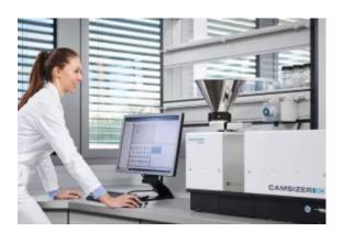
This technology ensures that the true size and shape values are recorded. Especially for the length measurement of stretched particles (e. g. extrudates) this is a decisive advantage compared to conventional 2D particle analysis, where the particles are captured in arbitrary orientation and do not show their "true"
