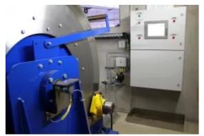
INGSPANN offers a wide range of drum and disc brakes for use in the drivetrains of belt conveyor systems and various system and monitoring modules that enables the implementation of intelligent complete solutions. (Image: Wiegand)
