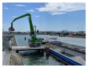
The 840 E unloads bulk material arriving at the Port of Edouard Herriot in Lyon and ensures efficient and fast supply to PRADIER's end customers and plants. (Pictures: ©SENNEBOGEN)
